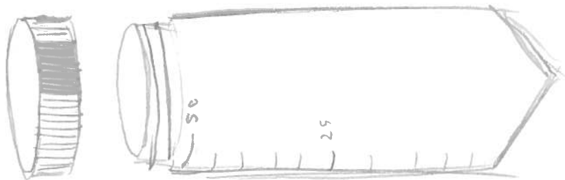
50 ml conical tube, screw cap. water-tight. often comes pre-sterilized.
