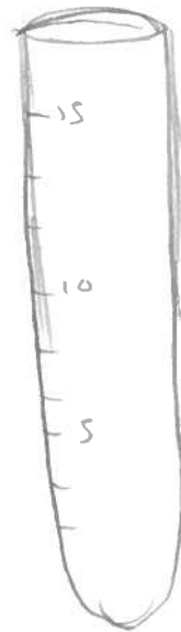
15 ml "falcon" culture tube. Often comes pre-sterilized, lid is not air or water tight, and snaps on
