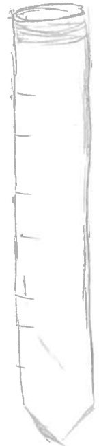
15 ml conical. Screw-on water-tight cap. often comes pre-sterilized.
